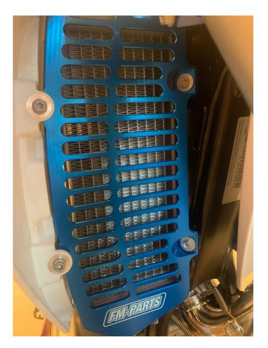
Make sure that the side of the radiator is in the protection channel
